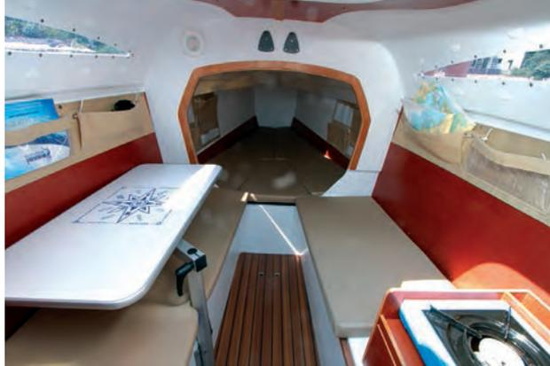
The volume is limited, but there are four good berths, a multi-purpose table, a galley unit and stowage space.
