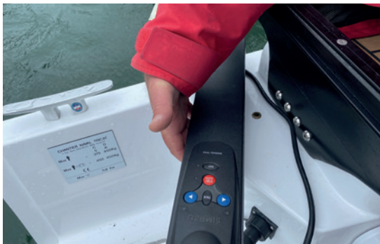
▲ A second mounting cup, further out, allows the autopilot to be stowed flat, away from the helm. The mounting cup visible in this picture is the one that holds the pilot when it's in use.
