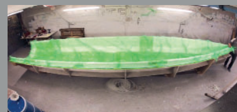
Tricat 20 infusion-built central hull
