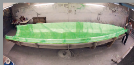
Tricat 25 EVO infusion-built central hull
