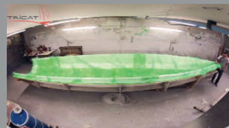
Tricat 6.90 infusion-built central hull
